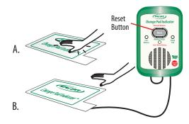
Test the system. (A) Put pressure on the sensor pad to activate the pad and the fall monitor. The fall monitor will beep two times to indicate that the sensor pad and the fall monitor are in use. The "Status" light will blink while pressure remains on the pad. (B) When pressure is removed, the fall monitor will sound the alert tone. Press the Reset button to silence the alert.
