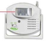
The pager will sound the alert tone when the infrared field is interrupted.
