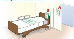
Mount the TL-2016 transmitter out of resident's reach if you are using an external device. (A) When using the Nuse Call" feature, mount the transmitter within the resident's reach. (B) Mounting hardware is included for bed or wall mounting.
